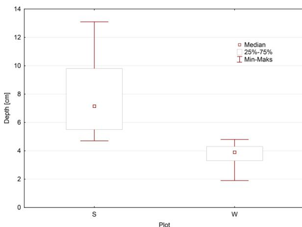
Fig. 4. Depth of soil disturbances
