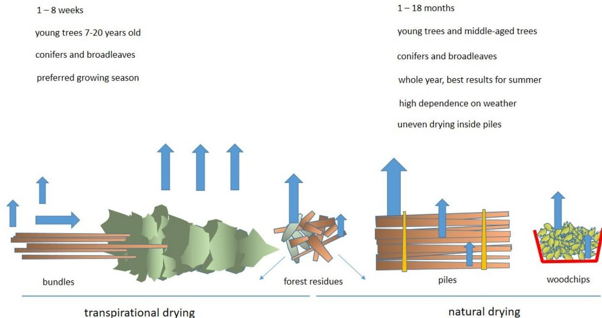
Figure 1. Scheme of natural drying methods.
